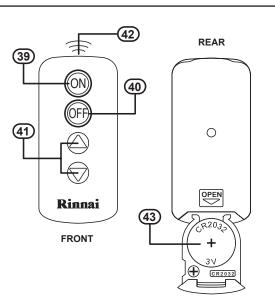
ONLY use the specified CR2032 3V battery for the remote control
