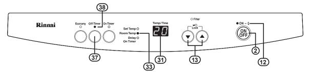
To operate, press the Off Timer button ③. The Off Timer indicator ③ will illuminate and the Combustion indicator ④ will be illuminated red to confirm that the heater will continue operation until the Delay 'off' time period has passed after which it will stop. The Delay Off time is 60 minutes. When this time has passed, the heater will automatically stop operation and the Off Timer indicator ③ will flash.
